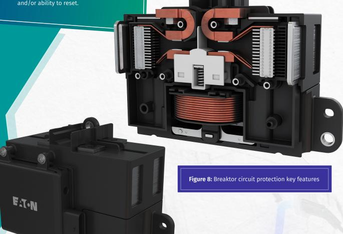
In normal switching operation, the driver coil closes the contacts powered by a 12V supply to switch the device on and falls back into off-mode when the supply voltage drops off.
