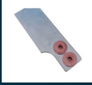
Figure 13: Cu Nut welded on Al bus bar with Telsonic Torsional welder SONIQTWIST® (APTIV\_NA Congress Presentation)
