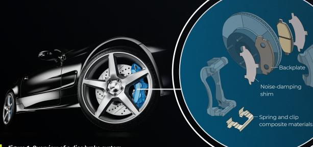
Figure 1: Overview of a disc brake system. The brake pad consists of friction material, a backplate, and an anti-noise shim.
