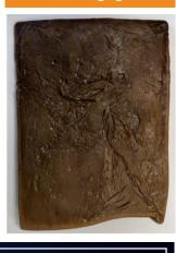
Figure 4B: Xydar® G-330 HH after 400 °C for 30 Minutes
